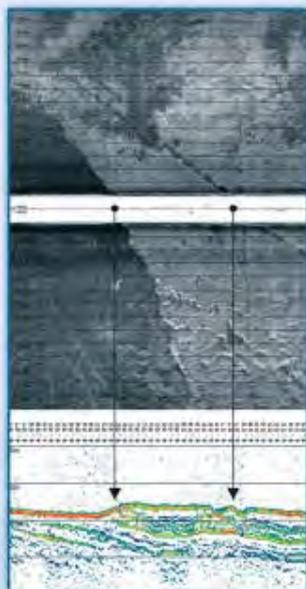
◀ Side Scan Echo Plot with simultaneously recorded Sub-bottom Echo Plot (SSS: 410kHz, SBP: 8kHz)
