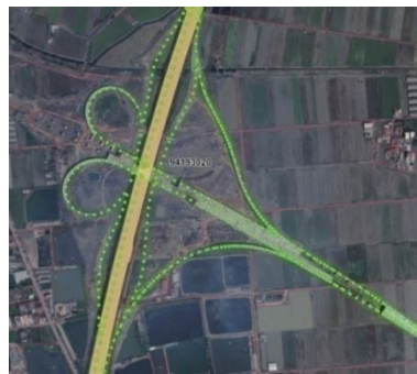
b. Existing road data overlapped with MMS data
