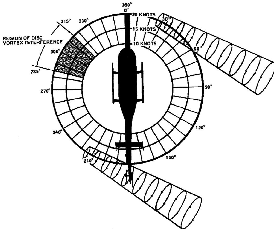
FIGURE 1. MAIN ROTOR DISC VORTEX INTERFERENCE
