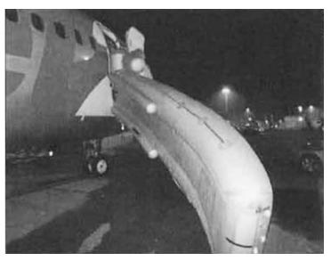
AAIB investigator say there were no mechanical problems with the Right front evacuation slide that twisted when deploying.
