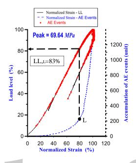
Fig. 5. Identification of localization by AE accumulated curve with respect to loading history (T<sub>max</sub> = 25 °C-1).
