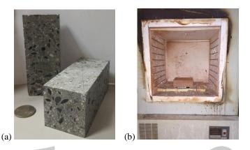
Fig. 1. Fire-damage concrete specimen preparation: (a) concrete specimen (b) high temperature oven.
