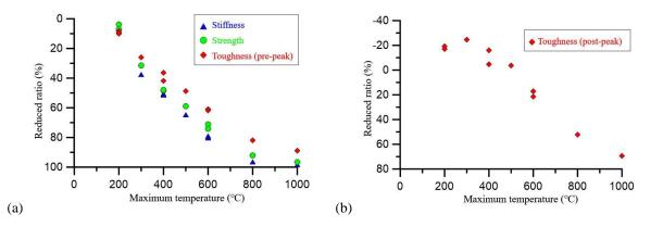
Fig. 4. Effect of fire temperature on stiffness, strength, toughness at pre-peak and toughness at post-peak.
