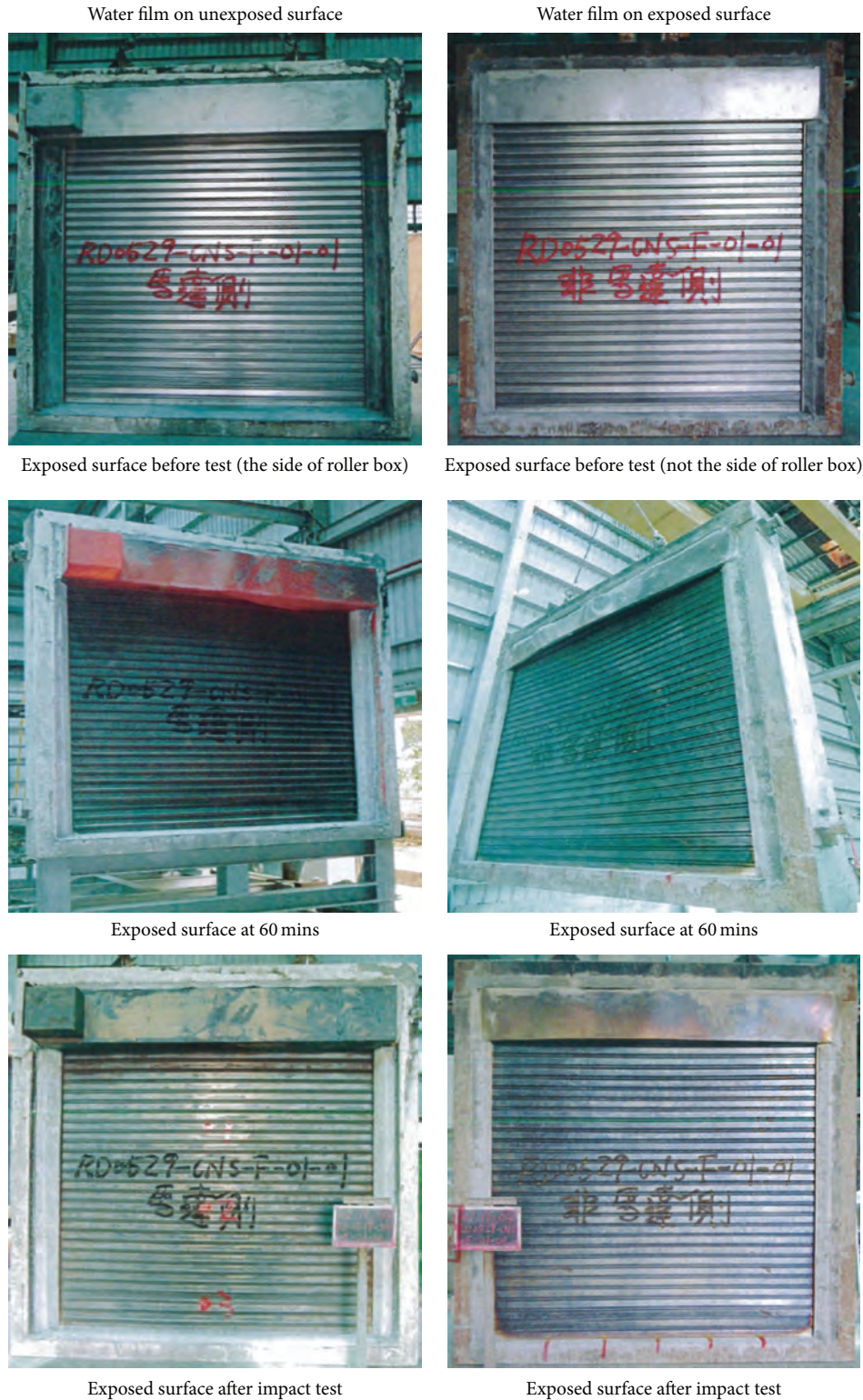
FIGURE 13: Exposed surface before heating test, at 60 mins, and after impact test with water film on exposed/unexposed surface.
