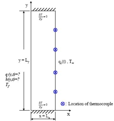
Fig.2 Schematic geometry of the present problem
