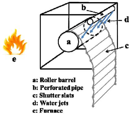
Fig. 1 Schematic of water film system
