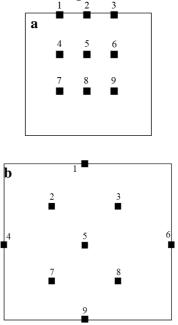
Fig. 1 Thermocouple positions on the (a) small-scale test and (b) full-scale test.
