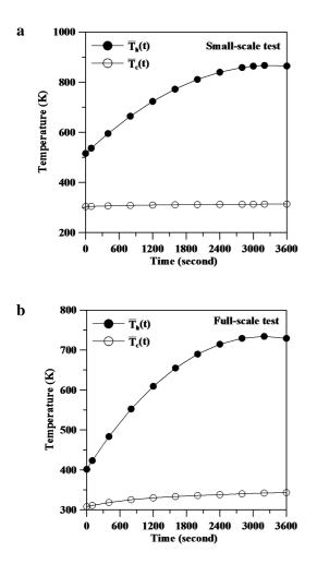
Fig. 5 History of the surface temperature on the hot  $\overline{T}_{h}(t)$  and cold surface  $\overline{T}_{c}(t)$  of the (a) small-scale test, (b) full-scale test.
