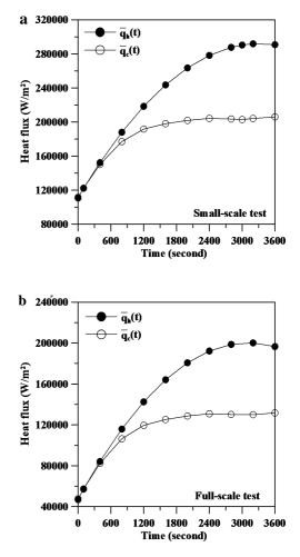
Fig. 4 History of the total incident heat flux on the hot  $\overline{q}_{h}(t)$  and cold surface  $\overline{q}_{c}(t)$  of the (a) small-scale test, (b) full-scale test.
