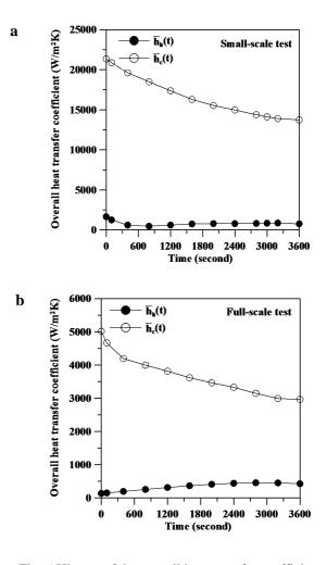
Fig. 6 History of the overall heat transfer coefficient on the hot  $\overline{h}_h(t)$  and cold surface  $\overline{h}_c(t)$  of the (a) smallscale test, (b) full-scale test.
