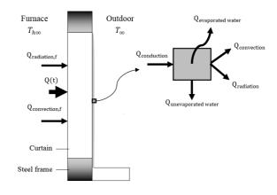
Fig. 3 Heat transfer mechanism on the fireproof curtain with down-flowing water film on the cold surface.
