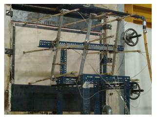
Fig. 4 Photograph of temperature measurement framework with thermocouples installed.
