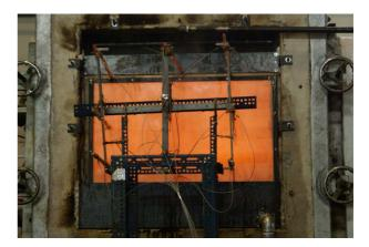
Fig. 8 Photograph of fireproof curtain with water film during test.
