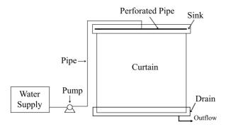
Fig. 5 Schematic of water film system.
