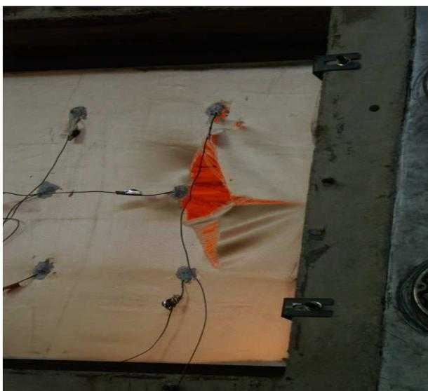
Fig. 6 Breakdown of fireproof curtain without water film.
