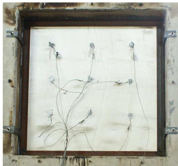
Fig. 3 Photograph of thermocouples attached on curtain.
