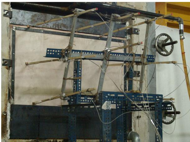
Fig. 4 Photograph of temperature measurement framework with thermocouples installed.
