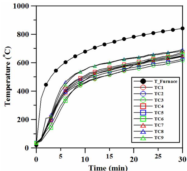
Fig. 7 Temperature distribution on the unexposed surface of fireproof curtain without water film.
