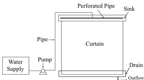
Fig. 5 Schematic of water film system.
