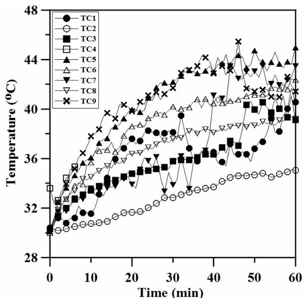
Fig. 9 Temperature distribution on the unexposed surface of fireproof curtain with water film.
