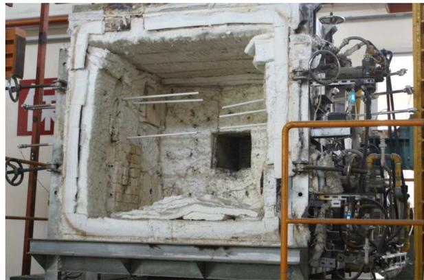
Fig. 1 Photograph of refractory furnace.
