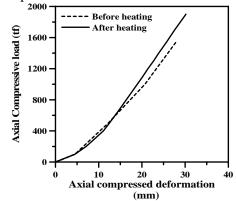
Fig. 12 Axial deformation of Spec. CFBC-1 before and after fire.
