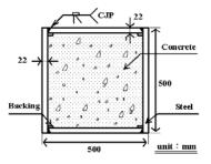
Fig. 7 Cross section of the specimens.
