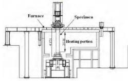
Fig. 9 Sketch of the furnace and test setup.
