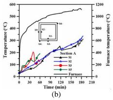
Fig. 13 Measured temperatures at cross section A of Spec. CFBC-2
