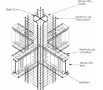
Fig. 1 The combination of steel and reinforced steel.
