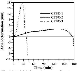
Fig. 17 Axial deformation versus fire time.
