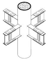
Fig. 5 Combination of round concrete-filled tubular column with steel beams.
