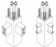
Fig. 2 The combination of cross-shaped encased SRC columns and SRC beams or steel beams.
