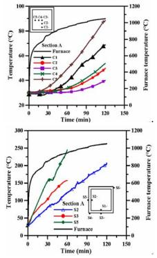
Fig. 10 Measured temperatures at cross section A of Spec. CFBC-1
