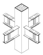
Fig. 4 Combination of square concrete-filled tubular column with steel beams.
