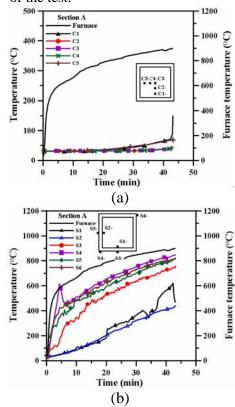
Fig. 15 Measured temperatures at cross section A of Spec. CFBC-3
