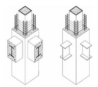
Fig. 3 Combination of encased concrete-filled SRC columns with SRC beams or steel beams.
