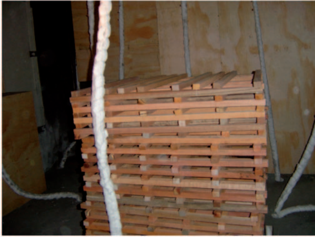
Figure 5. A full-size wood crib.
