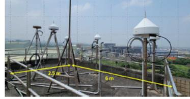
Fig. 1 The antennae of physical receivers in ensemble are located in a 2.5 m × 6 m area
