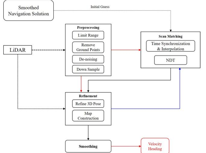
Fig. 2. Overview of proposed 3D NDT LiDAR-SLAM
