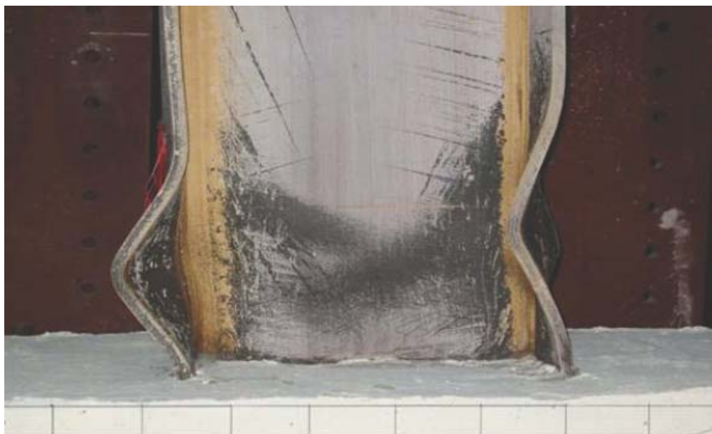
(c) 試體SRC4-VR0.82位移 12\Delta y 時(Story Drift Angle \theta_t = 5.73\% )
