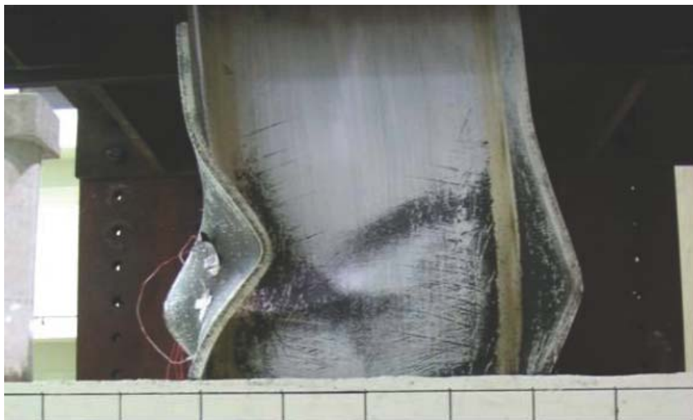
(a) 試體SRC2-VR1.15位移 13\Delta y 時(Story Drift Angle \theta_t=6.20\% )
