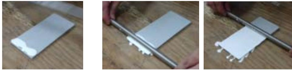
(a)將塗料倒於試片一端 (b)微施壓力均速拉動塗佈器(不可轉動)
