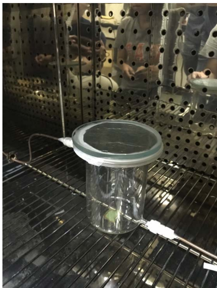
Florisil®溶劑萃取法檢測建材(塑膠地板)逸散塑化劑
