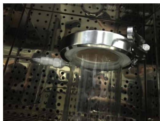
Florisil®溶劑萃取法檢測建材(塑膠地板)逸散塑化劑
