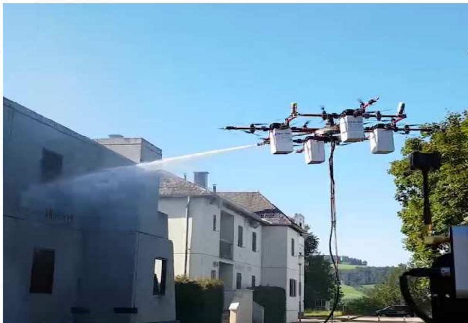
圖 4- 6 Aerones firefighting drone
