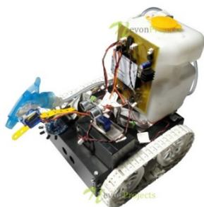
**圖 4- 8 Arduino Based Autonomous Fire Fighting Robot**
