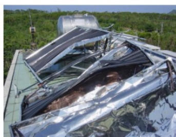
Figure 1.1.1 Damaged solar collectors (after Chung et al. 2008)
