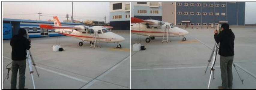
圖 2-11 Lever arm 量測作業照-P68C-TC
