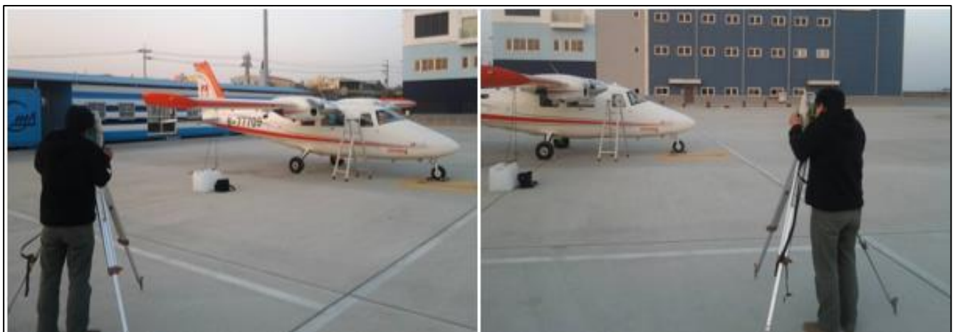
圖 2-17 Lever arm 量測作業照-P68C-TC
