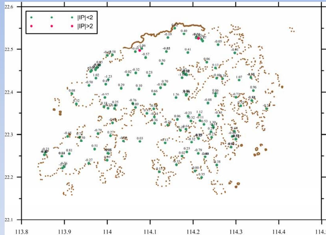
The internal precision of quasi-geoid model II (unit: cm)
