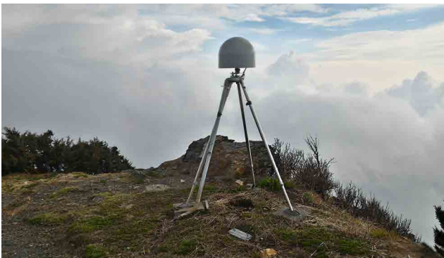
▲ 臺灣地區最高之玉山北峰 GNSS 衛星連續觀測站 The GNSS satellite continuously operating reference station on the north peak of Mt. Jade.
