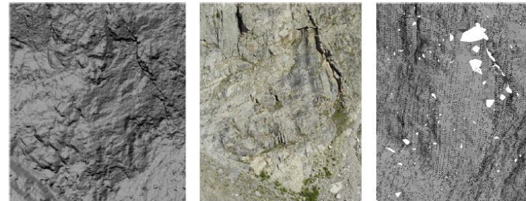
Left: Derived surface model from image matching, Middle: Zoom-in of an UAV-image, Right: Point cloud of Helicopter-based LiDAR projected on the derived surface model.
