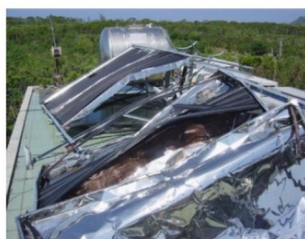
Figure 1.1.1 Damaged solar collectors (after Chung et al, 2008)
