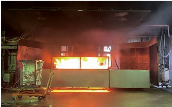
Car fire and sprinkler fire-extinguishing experiment in simulated parking space (left: simulated car body burning experiment, right: actual car body burning experiment)
