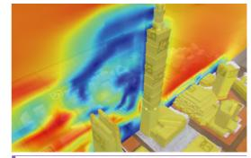
Flow Field Visualization Results by CFD Simulation and AR Software
