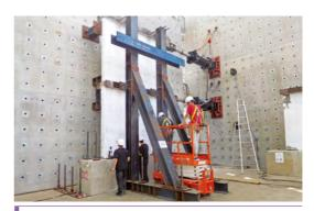
Multi-Unit Steel Tube and Cyclic Testing of Mesh Walls
